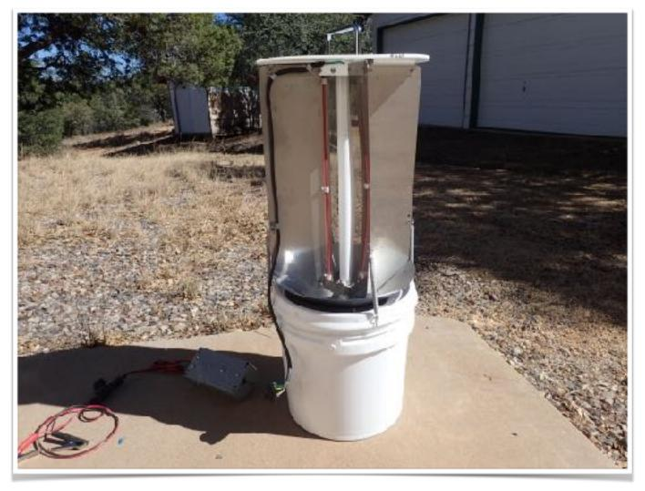
A portable light trap, note the alligator claps at the lower left of the photo. Such units are often powered by car batteries or in some cases, special purpose batteries.
