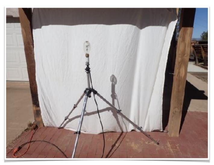
UV Lamp and Sheet - Moths are attracted to the light and settle on the sheet.
