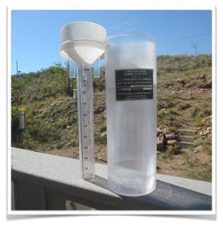
In the colder times of the year, when frozen precipitation is anticipated, the funnel and collection tubes are removed from whichever gauge is being used and the precipitation is collected in the larger cylinder. The cylinder is then moved indoors just before the reporting time, the precipitation is allowed to melt completely, and the liquid is poured into the collection tube for a measurement.
